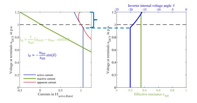
Figure 31: Active and reactive current of an inverter behaving as voltage source if no current limits apply.
