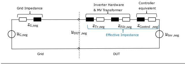
Figure 41. Test system for testing unbalanced voltage step.
