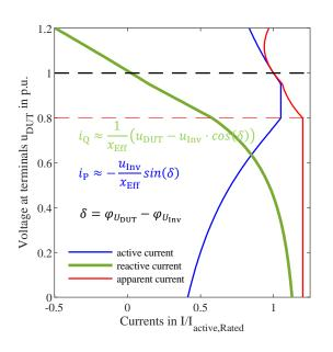
Figure 6: Active and reactive current of an inverter with current magnitude limitation.
