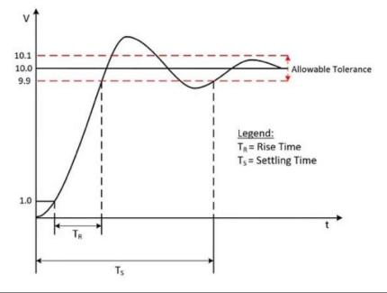
Figure 5: Definition of rise time and settling time
