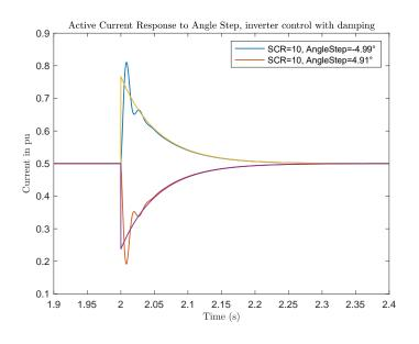
Figure 4: Analytical calculation of phasor and instantaneous values of active current change with angle step by +- 5° at the grid voltage source. See also Annex B
