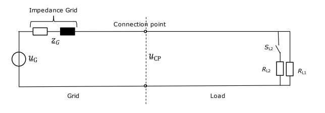
Figure 18: Simple grid and load equivalent for estimating a voltage angle change following a load change.
