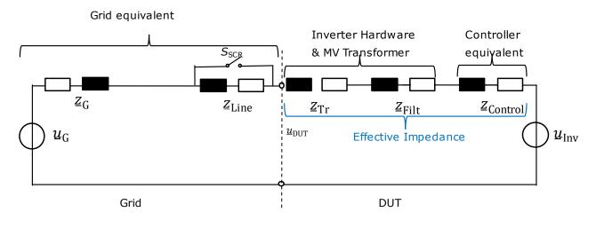
Figure 10. Simple grid equivalent consisting of a grid equivalent, unit MV transformer, inverter filter and control impedance for testing voltage angle steps.
