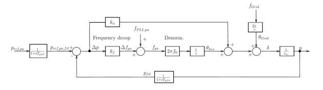
Figure 13 Reference implementation of a GFM active power control loop.
