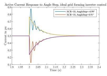
Figure 24: Active current change with angle step by  $\pm$  4.9° at the grid voltage source with simplified grid forming control according to Figure 14. The yellow and pink lines show the phasor based calculation.
