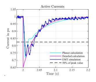
Figure 26: Active current change following voltage angle change by 5° at the terminals of the unit at rated power. Comparison of ideal and simulated response to voltage angle change.
