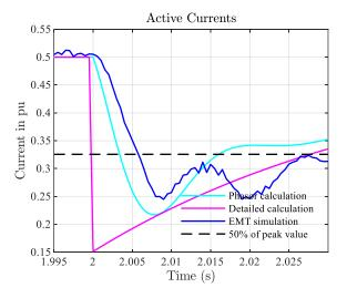
Figure 29: Detailed view of active current change following voltage angle change by 5° at 50% rated power.
