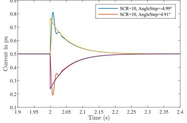
Figure 25: Active current change with angle step by  $\pm$  4.9° at the grid voltage source with inverter control and additional damping.
