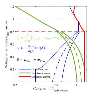
Figure 8: Active and reactive current of an inverter with current magnitude limitation, including an allowed band for the current reference of 90% of the theoretical value.
