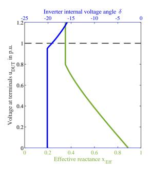
Figure 7: Corresponding values of voltage angle  $\delta$  (green line), and effective impedance  $x_{Eff}$  (blue line) for an inverter with current magnitude limitation. The internal voltage of the inverter remains constant.
