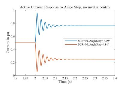
Figure 20: Active current change by  $\pm$  25% resulting from a change of grid voltage angle.
