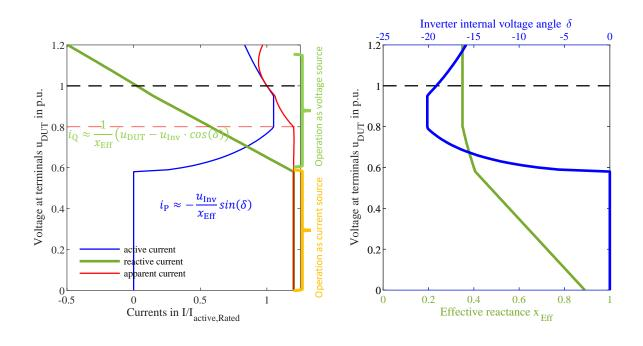
Figure 35: Active and reactive current of an inverter with voltage control and reactive current priority in a typical configuration for solar plants.
