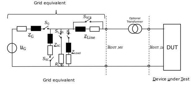
Figure 9. Test setup for evaluating the DUT performance.
