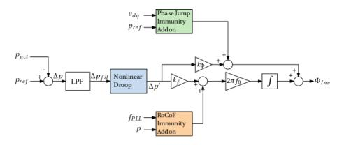
Figure 15 Additions to basic control structure for protection against overload conditions during grid.
