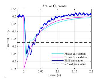
Figure 28: Active current change following voltage angle change by 5° at the terminals of the unit at 50% rated power. Comparison of ideal and simulated response to voltage angle change.
