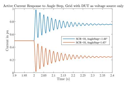
Figure 22: Active current change by  $\pm$  25% resulting from a change of grid voltage angle with damping and without inverter control.
