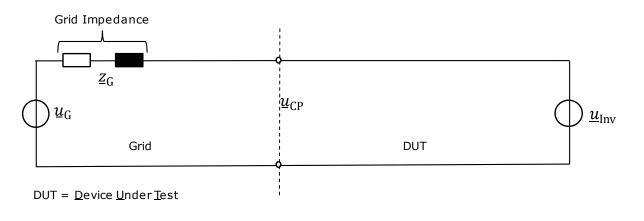
Figure 19:Simple grid equivalent consisting of a grid equivalent and an idealised DUT.
