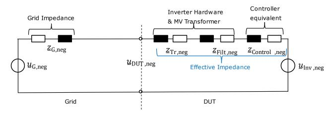
Figure 3: DUT negative sequence controller equivalent representation for evaluating the response to grid disturbances.
