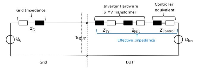
Figure 23: Simple grid equivalent consisting of a grid equivalent, unit MV transformer, inverter filter and control impedance.
