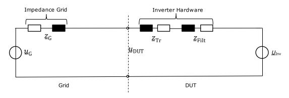
Figure 21: Simple grid equivalent consisting of a grid equivalent, unit MV transformer and inverter filter impedance.
