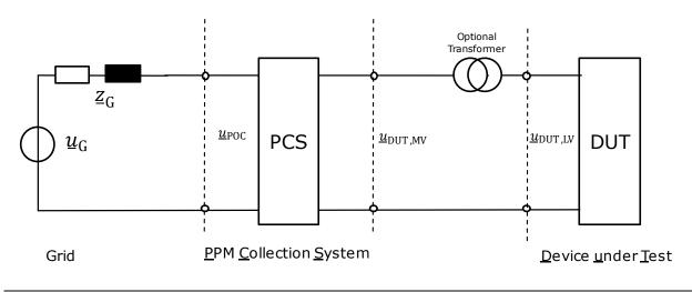
Figure 1: Definition of PPM PoC and unit terminals on medium and low voltage
