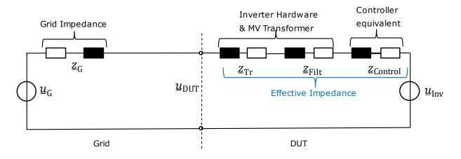
Figure 2: DUT positive sequence controller equivalent representation for evaluating the response to grid disturbances.
