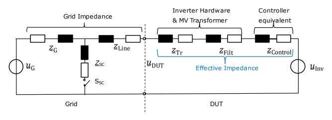
Figure 11: Simple grid equivalent consisting of a grid equivalent, unit MV transformer, inverter filter and control impedance for testing voltage amplitude steps in simulation or measurement.
